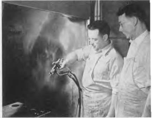
Lacquer to produce the distinctive GR crackle finish is being sprayed on a panel by H. J. Goodall, while T. Palmer, foreman of the plating and finishing department, looks on.
