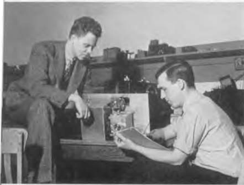
Dr. D. B. Sinclair, Engineer (left), and C. A. Woodward, assistant, specialists in high-frequency measurements, are shown working on a new impedance bridge for use at high frequencies.
